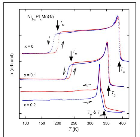
Temperature dependence of the permeability of the Ferromagnetic Shape Memory Alloys Ni<sub>2-x</sub>Pt<sub>x</sub>MnGa (x= 0, 0.1, 0.2).  $T_{\rm M}$ 's (martensitic transition temperature) are increased and  $T_{\rm C}$ 's (Curie temperature) are decreased with the Pt substitution, x.
